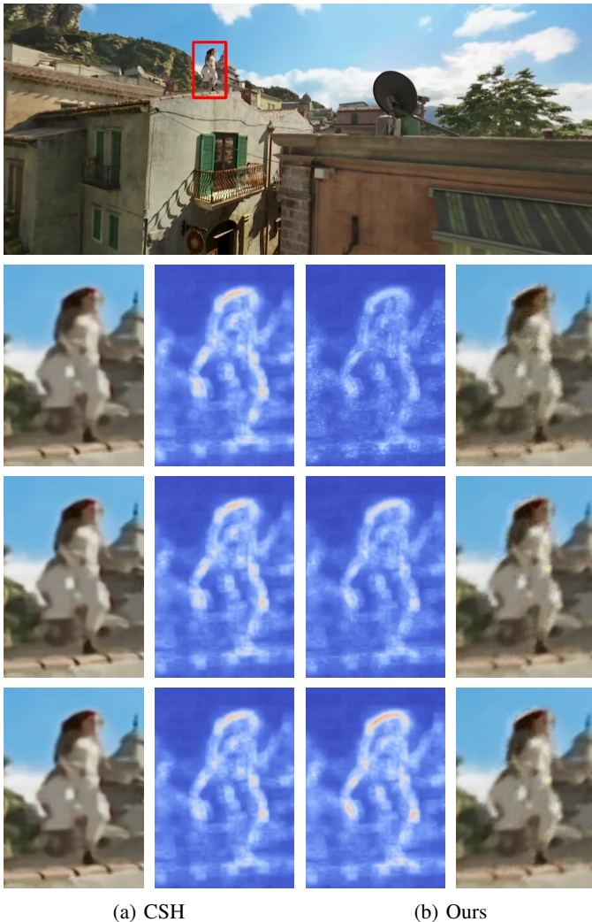
Fig. 5: Accuracy of generated fields and their respective reconstructions. Top row: Original image. Second row: Reconstruction as well as the Euclidean error of the highlighted area after 3 iterations (CSH) and with PCA 5 ( opencl ). Third row: 5 iterations (CSH) and PCA 10 ( opencl ). Fourth row: 10 iterations (CSH) and PCA 20 ( opencl ).
