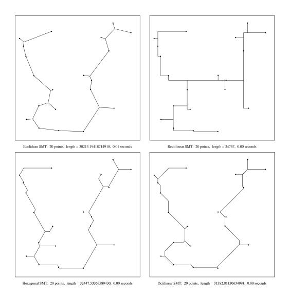
Figure 1: SMTs for the same set of terminals under different metrics (output from GeoSteiner).
