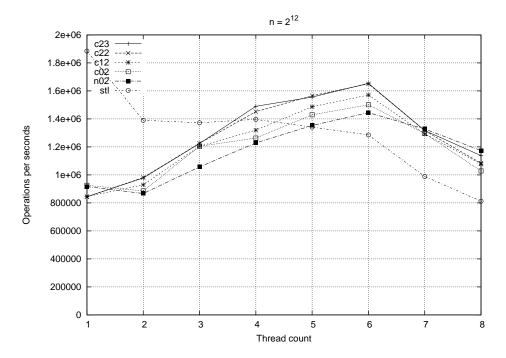
Figure 5.8: *Operations per second:* The STM version scales reasonably up to six threads, but cannot outperform the STL-version. There is some advantage to using a good layout. In this particular instance the n02 performs worse than the c02 setup.
