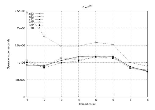
Figure 5.10: *Operations per second:* The STM version does not scale well. The different layouts perform about the same. There is considerable variations in the runtime from run to run (not shown).
