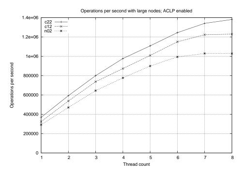
Figure 5.12: *Operations per second:* Large nodes are used and the ACLP feature is enabled; two node slots can fit in two adjacent cache lines. The c22 layout is significantly better than the others.
