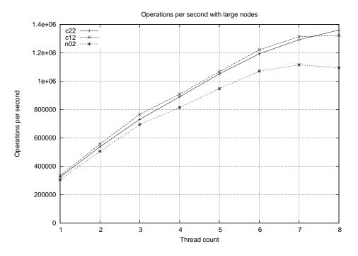
Figure 5.11: *Operations per second:* Large nodes are used; only one node slot can fit in a cache line with the handle. The c12 layout performs best, though the c22 layout is close.
