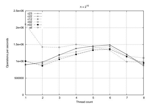
Figure 5.9: *Operations per second:* The STM version does not scale well. There is a small advantage to using a good layout.
