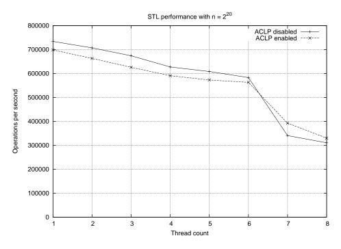
Figure 5.13: *Operations per second:* Comparing the STL runs with and withour ACLP enabled. Small nodes are used. ACLP is a disadvantage with less than seven threads.
