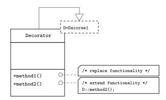
Figure 10. An alternative generic version of the decorator design pattern. The class Decoree1 is illustrated in Figure 9.
