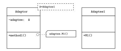
Figure 11. The generic version of the adaptor design pattern.
