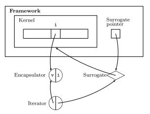
Figure 5. The surrogate mechanism.
