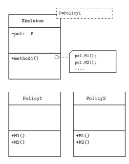
Figure 13. The generic version of the template-method design pattern.
