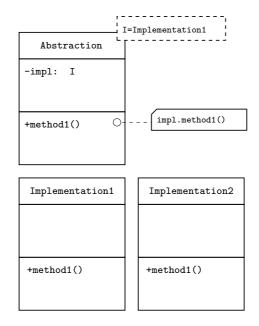
Figure 7. The generic version of the bridge design pattern.
