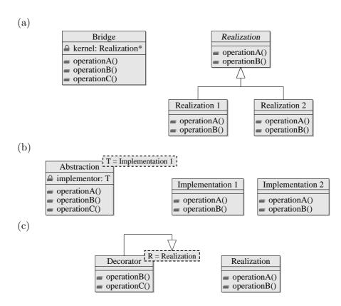
Figure 1. (a) The conventional bridge pattern, (b) the generic bridge pattern, and (c) the generic decorator pattern.
