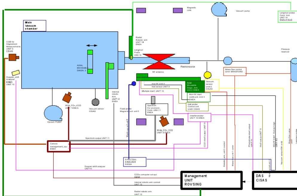
Figure 2. Schematics of the HPH.com Engineering model experiment.
