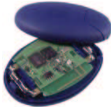
Figure 4: Bluetag. Bluetooth based smart-tag.
