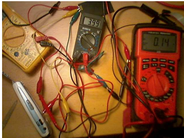
Figure 6.5: Experimental setup for the p800. Note the total system power consumption of 3.99 V * 0.14 A = 559 mW for a running JVM. The measurement instrumentation is placed between the battery and the phone.
