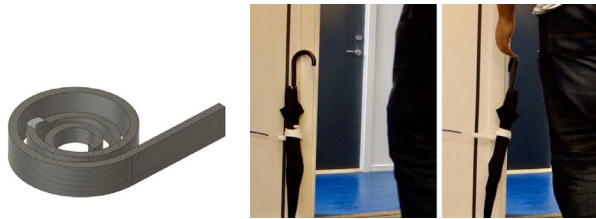
Figure 5.7: Left: The 3D model of an umbrella pusher created by our plug-in and edited in CAD software. Middle: The umbrella pusher is holding an umbrella. Right: On a rainy day, the umbrella pusher slightly unbends and pushes the umbrella towards on the way of users to remind to take the umbrella. The central part of it unbends less and still holds the umbrella.
