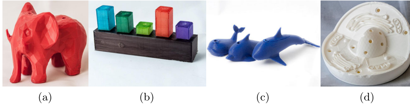
Figure 4.1: Example Blowhole applications. The elephant (4.1a) has six holes (one on the head, one on the back, one on each foot) which, when blown into, activate text-to-speech with different elephant facts. Each bar in the bar chart (4.1b) triggers a readout of the quantity, and can be moved to represent different data. The sperm whale, dolphin, and orca (4.1c) each produce a different tone to trigger videos of those animals. The cell model’s blowholes interact with a quiz program to test knowledge of its components (4.1d).
