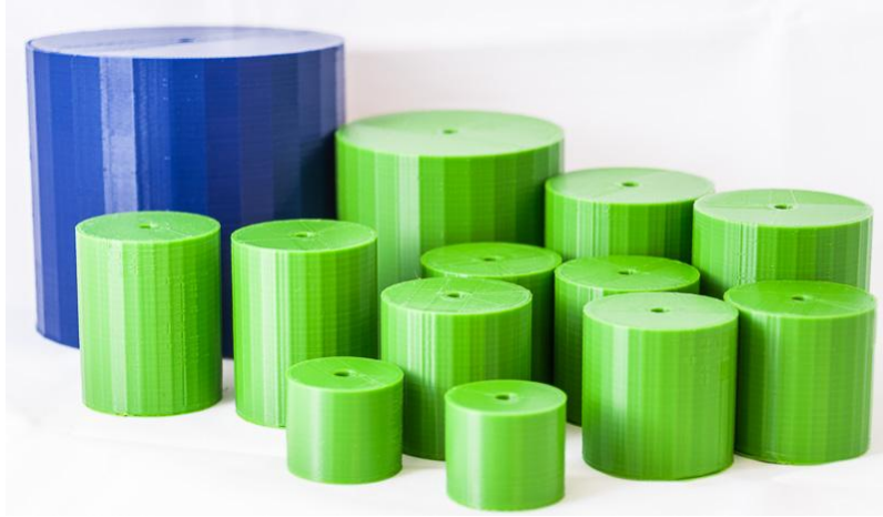
Figure 4.3: A subset of our test cylinders with varying cavity volumes and tube lengths.
