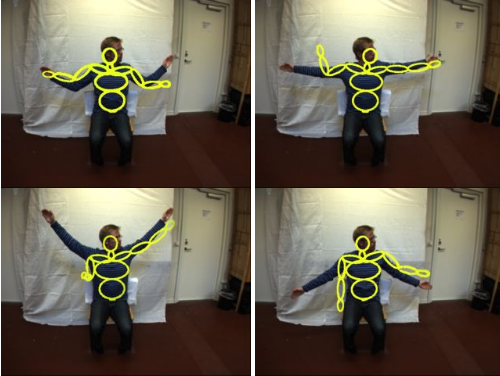
Figure 14: Traditional motion estimation in full pose space using 100 particles. Notice that the superimposed figure loses track of the person in the image.
